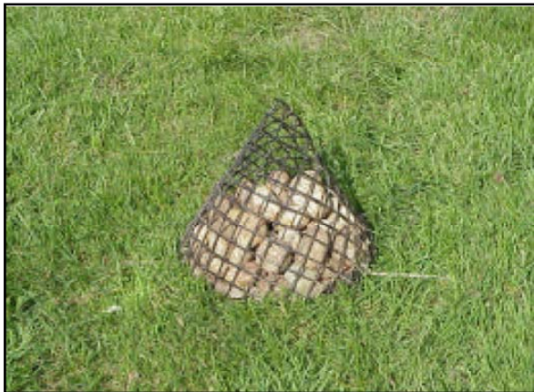
Remote-retrievable rock-filled cone and retrieval funnel for sampling non-wadeable rivers
