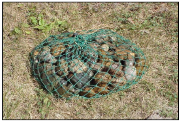
Rock-filled riffle bag for sampling streams less than 10 cm deep
