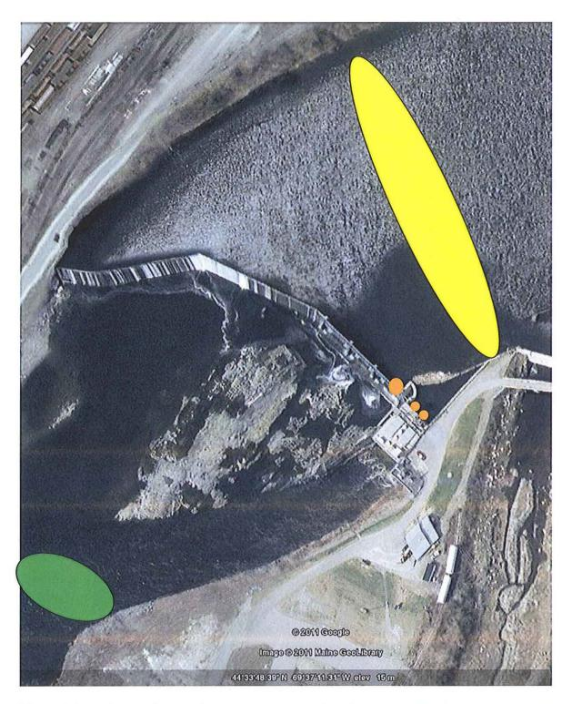
Figure 1. Locations and approximate coverage area for telemetry monitoring stations 1 (yellow), 2 (orange) and 3 (green) at the Hydro Kennebec Project.
