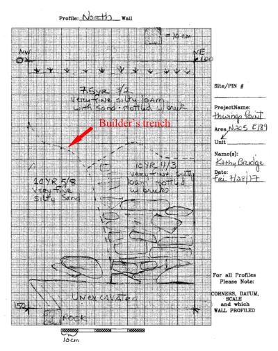
**Figure 8.** Profile of the north wall of N205 E189 showing rock wall and probable builder's trench noted. It can be seen that the rock wall was build against the wall of the builder's trench.
