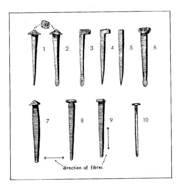
**Figure 13.** Example of nails showing hand-forged nails at top and three cut nails and a wire nail (far right) at bottom. (After Noël Hume 1969: 253.)
