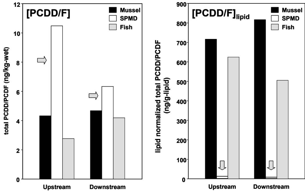
Figure 4. Total dioxins and furans in caged mussel tissues, SPMDs, and fish from upstream and downstream stations, and on a lipid-normalized basis.
