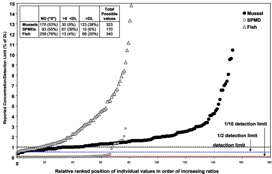
Figure 5. Percent of values >0 compared distribution detection limits (DL) for caged mussels, SPMDs, and fish. For non-detected (ND) values, a "0" was used to represent reported concentration. Total possible values = number of samples analyzed x 17 congeners. Graph does not show percent of values that were non-detects.
