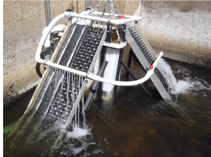
**Type:** full-height lift with ramp trap, pumped supply
