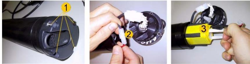
The Aquadopp Profiler is shipped with a battery pack installed in the pressure case, but disconnected. The following procedure outlines how to connect the battery pack or to install a new one.
