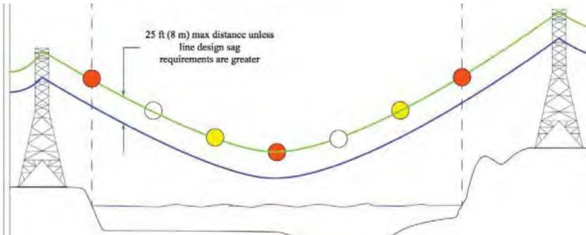
**Fig. 4:** A diagram of unlit marking balls.<sup>7</sup>
